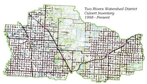
Locations of culverts within the Two Rivers Watershed District. Culvert sizing can be an important tool in reducing flooding and erosion.
